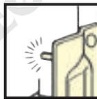
\* PULP version has pin that prevents spreading of the door from frame
